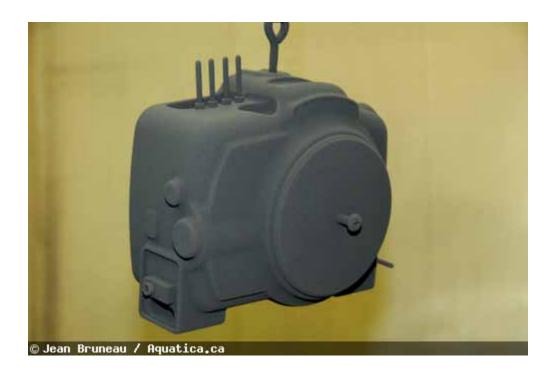
This skin has a much harder finish than the conventional method of painting and is exactly what the salt water environment requires. Ok, so now you got me, in the beginning I stated that housings did not come out of an oven; well they do at some point!
