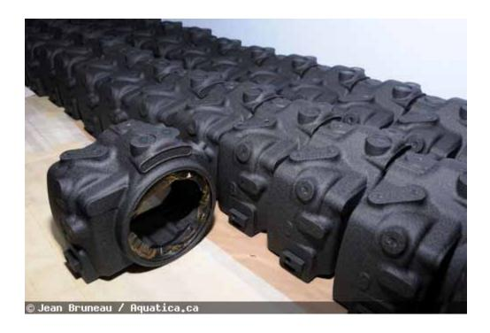
Once the housings have cooled down, they are brought back to the assembly room. The masking material is removed in preparation for the attaching and painting of the different logos and operational labels. Aside from the company logo that is attached with a waterproof bonding material, all other symbols or text on the housing are pad printed with a highly resistant paint. It was found that applying stick-on labels just did not last long enough in the harsh underwater environment.
