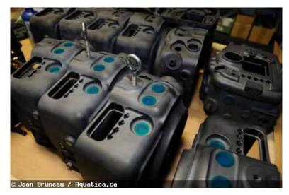
Once prepped up the housings are transferred to the paint shop. For a layer of protection we use a powder-coated treatment. This coating is a highly resistant finish that is applied through an electrostatic process and then baked.
