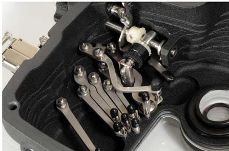
The Austenitic, 304 series of stainless steel alloy used by us, contain a maximum of 0.08% carbon, a minimum of 20% chromium and sufficient nickel and/or manganese to retain its austenitic structure at all temperatures from the cryogenic region to the melting point of the alloy. Every shaft is polished to a mirror finish, calibrated and its operation validated by the quality
