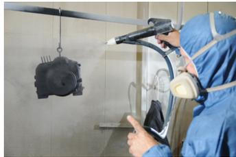
This extra layer of protection comes in the form of a Polyester powder coating that is sprayed on the housing shells with an electrostatic process, this robust coating, once cured for 15 minutes at 350F/177C, will resist a direct impact of up to 160 in-lb (as per specification ASTM D2794), it is certified to resist yet another straight 1,500 hours of being sprayed with salt water and to meets or exceed the for environmental resistance to the elements.
