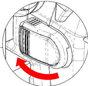
*NOTE: The latch is shown in its final locked position.*
