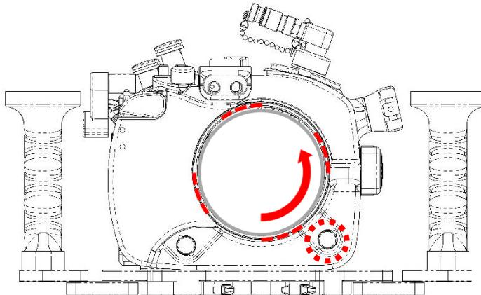
**STEP 2:** Carefully pull the port or extension ring out of the housing.
