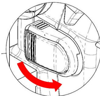
*NOTE: The latch is shown in its initial locked position.*
