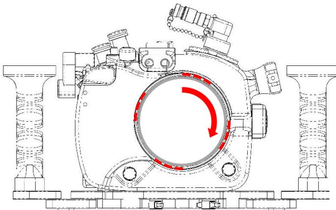
**STEP 4:** Push with even force on both sides of the port or extension ring until you feel it snap into place. Make sure the bayonet is completely inside the housing.
