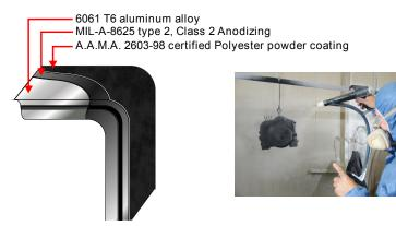
This extra layer of protection comes in the form of a Polyester powder coating that is sprayed on the housing shells with an electrostatic process, this robust coating, once cured for 15 minutes at 350F/177C, will resist a direct impact of up to 160 in-lb (as per specification ASTM D2794), it is certified to resist yet another straight 1,500 hours of being sprayed with salt water and to meets or exceed the for environmental resistance to the elements.
