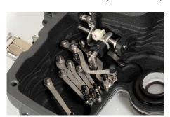
The Austenitic, 304 series of stainless steel alloy used by us, contain a maximum of 0.08% carbon, a minimum of 20% chromium and sufficient nickel and/or manganese to retain its austenitic structure at all temperatures from the cryogenic region to the melting point of the alloy. Every shaft is polished to a mirror finish, calibrated and its operation validated by the quality
