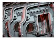
coating will have to resist a battery of torture, including a minimum of 336 hours being sprayed with a salt water solution, in the end, it will only get the stamp of approval if the anodizing coating show absolutely no signs of wear.
