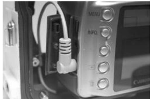
**Picture B: Trigger release cable position**
