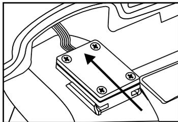
1- If using wired connection for the strobes, slide the housing's hot shoe connector onto the hot shoe base of the camera as seen in drawing at right.
