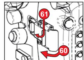
d) Always verify that the safety locking mechanisms (# 61) of the latches are properly engaged prior to entering water to avoid any accidental opening.
