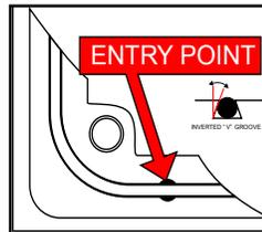
2- Once the O-ring is removed, it should be examined for damage. Check to make sure that the O-ring is free of nicks and cuts and that it retains its original round profile. O-rings that appear to be damaged should be discarded immediately and replaced with new O-rings.
